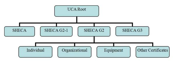
The length of UCA Root root key is 2048-bit. There are four sub-CAs under UCA Root-G2, including: (1) SHECA G2 is responsible for issuing the 1024-bit or 2048-bit certificate individual certificates, organization certificates, equipment certificates and other certificates with RSA algorithm, and is forbidden to sign SSL certificates. (2) SHECA, SHECA G2-1 and SHECA G3 no longer issue any subscriber certificates.
