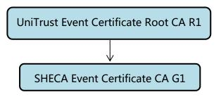
UniTrust Event Certificate Root CA R1 Root key is 4096-bit, under which is SHECA Event Certificate CA G1 acting as the only sub-CAs under UCA Root-G2, responsible for issuing intermediate certificate of 2048-bit with RSA algorithm.
